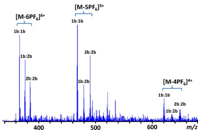
**Fig. 2** Portion of the electrospray mass spectrum (at  $t = 190$  min) showing the peaks corresponding to the loss of four, five and six  $PF_6^-$  anions of the  $M_3L_2$  cages [**1b** : **1b**], [**2b** : **2b**] and [**1b** : **2b**].
