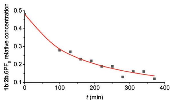
**Fig. 3** Relative concentration of cage [**1b** : **2b**] with respect to the total concentration of cages as a function of time (filled squares). The red line shows the fitting curve (Origin 7.0) obtained employing a second order rate law.
